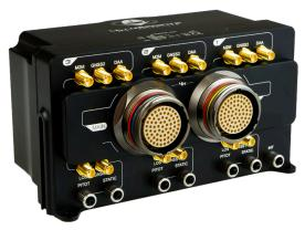
The Veronte Autopilot 1x is designed to control any unmanned vehicle: UAVs, multirotors, helicopters, airplanes, Hybrid VTOL, blimps ... as well as ground and surface vehicles, and many others.
